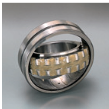
Sealed-type bearing after testing (unchanged from pre-test condition)
