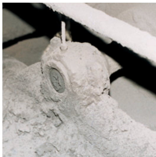
Bearing for pulley use (under actual operating conditions)
