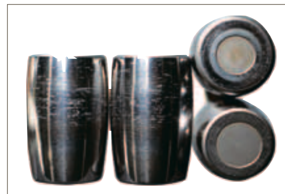
Fig. 35 Scoring on the Roller End Face
