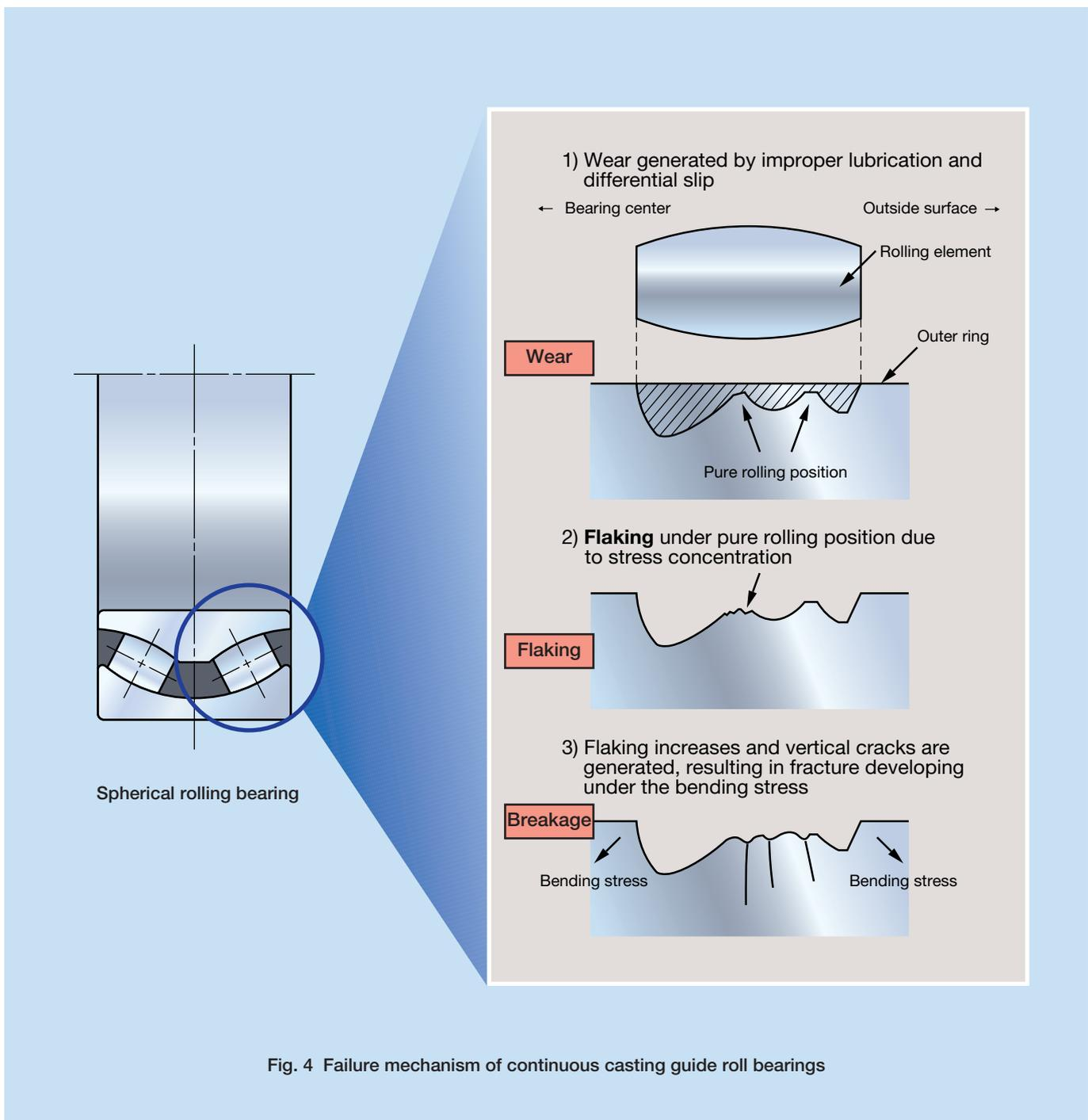
Fig. 4 Failure mechanism of continuous casting guide roll bearings
