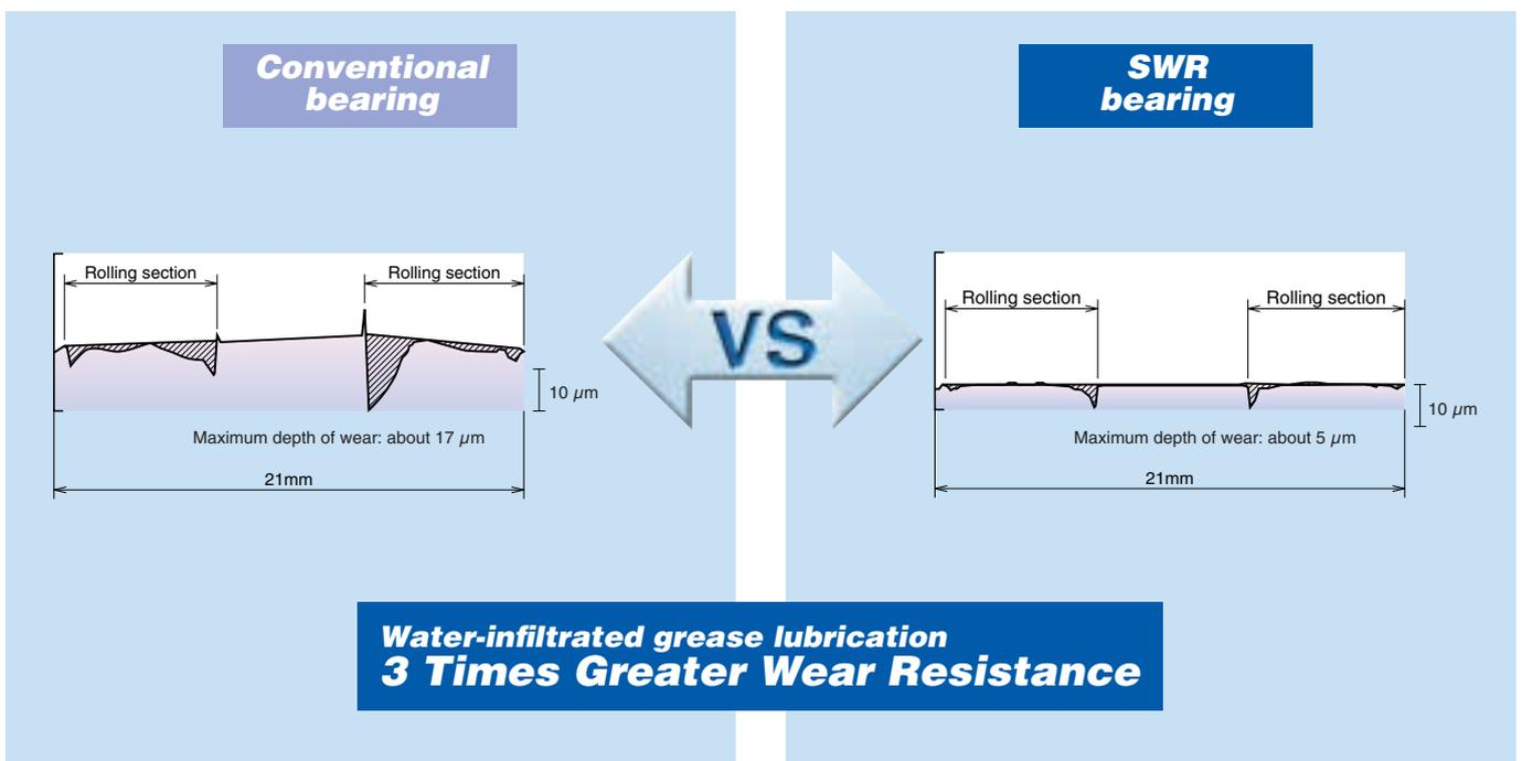
Fig. 5 Cross-section profile of the outer ring raceway after test (maximum loaded region)
